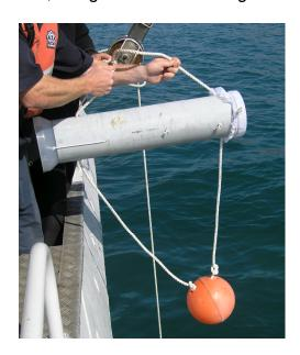
**Figure 9**. Example of IMR Light trap used in this study.
